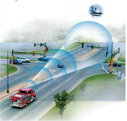
nicate with emergency vehicles when they are approaching an intersection. The SMARTDrive Multimodal Intelligent Traffic Signal system will selectively prioritize and notify all approaching emergency vehicles about which vehicle has the right-of-way. This will significantly improve efficiency and safety.
